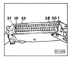
Contact assignment at connector for control unit –J220 (the contact assignment is identical to the socket assignment of the test box V.A.G 1598).
