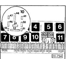
Test cable from contact 2 of the connector at the ACF valve to fuse –S24 for open circuit on the basis of CFD.
