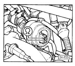
Connect hand-held multimeter V.A.G 1526 with auxiliary cables from V.A.G 1594 for resistance measurement to the idling stabilization valve.
