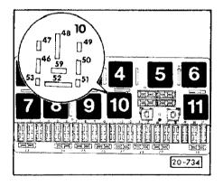
Test cable from fuse 25 to fuel pump relay -- 117 (replay position 10), contact 52, for open circuit on the basis of the CFD. Specification max.  $0.5 \Omega$ .
