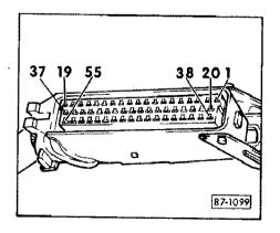
Rectify any short circuit or open circuit between contact 4 of the connector at the air mass meter and contact 25 of the connector at the Motronic control unit.
