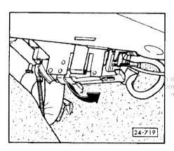
Wait at least 30 seconds after switching off the ignition before releasing and unplugging connector from the Motronic control unit.
