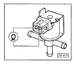
Connect hand-held multimeter V.A.G 1526 with auxiliary cables from V.A.G 1594 for resistance measurement to the solenoid valve for boost pressure limiting.
