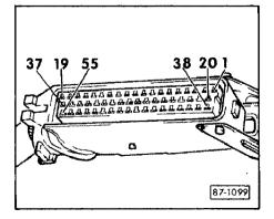
Rectify any open circuit or short circuit in the cables between the respective sensor coupling and the connector at the Motronic control unit, contacts 11/29, 30, 19.
