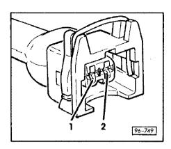
Test cable from contact 1 of the connector at the solenoid valve for boost pressure limiting to fuse 24 for open circuit on the basis of the CFD. Specification max. 0.5 Ω.
