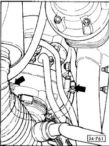
Earth connection for ignition coils at rear right of cylinder head cover.
